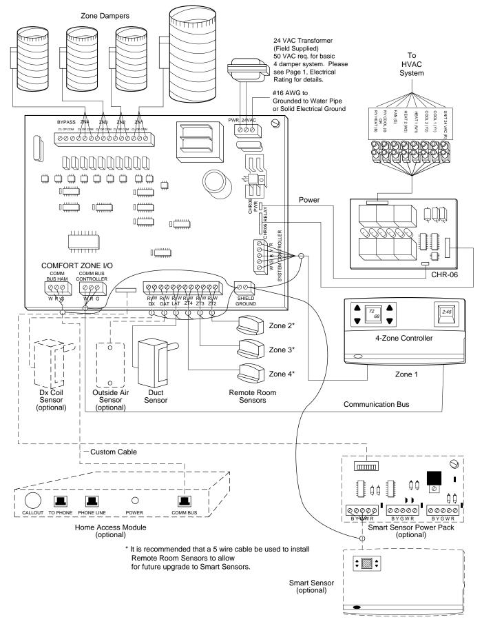
Fig. 16—Comfort Zone System Wiring Diagram
